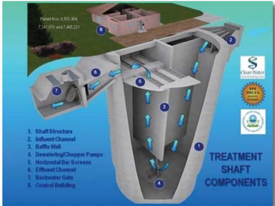
Figure 1. Patented Treatment Shaft Technology.
